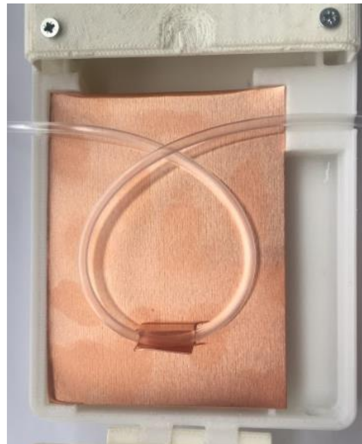
Figure 51 - Copper plate in the fluid warmer
