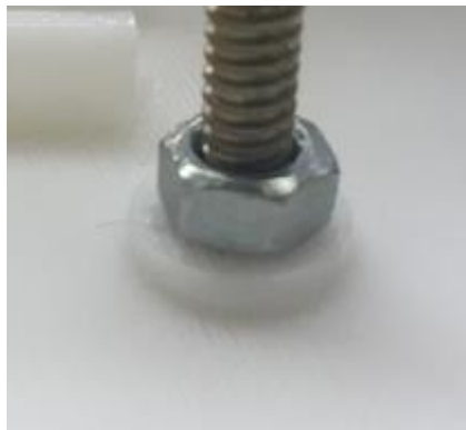
Figure 47 - Extra material at the base of the nut
