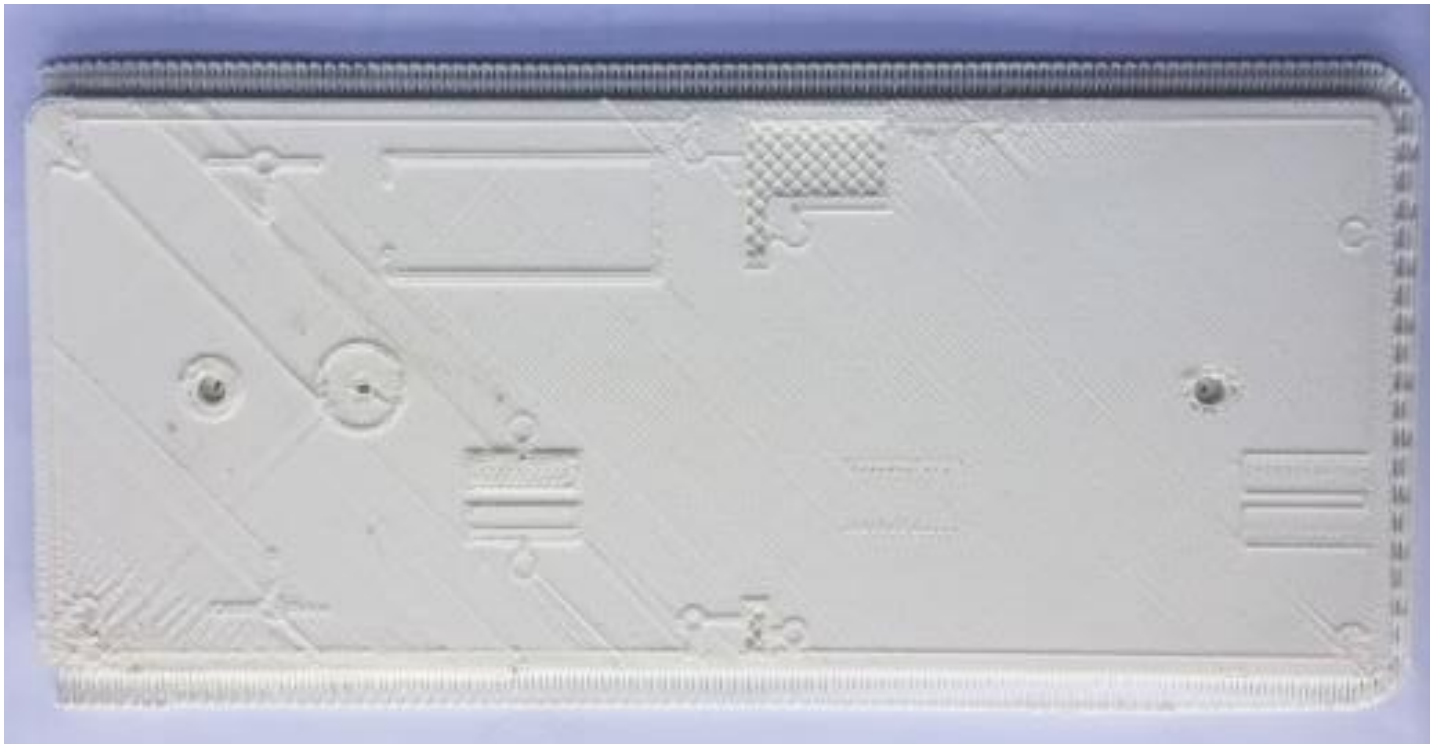
Figure 55 - 3D print that stopped due to power cut
