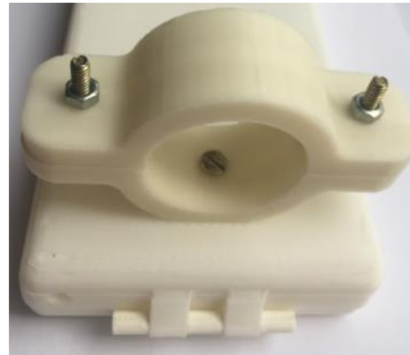
Figure 39 - IV stand holder on the back of the casing
